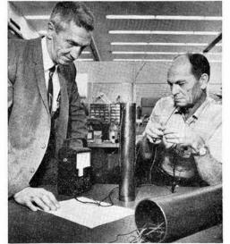
HEAT TRANSFER SPECIMENS are checked at the Laboratory by Frank D. Kite (9312), left, and O. A. Phelps (7125). The instrument is used in Project Pyro tests to gather heat transfer data for aerospace nuclear safety program.
